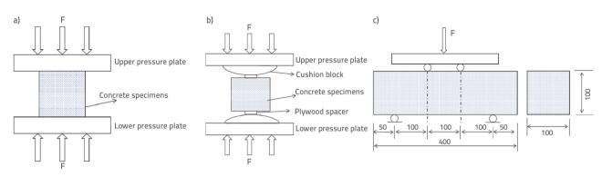
Figure 5. Schematic diagram of experimental loading: a) Schematic loading diagram of compressive test; b) Schematic loading diagram of splitting tensile test; c) Schematic loading diagram of flexural test
