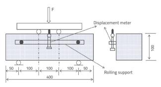
Figure 7. Flexural toughness test, specimen 100 x 100 x 400 mm
