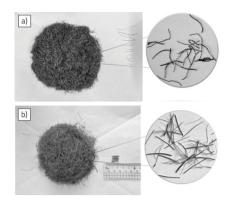
Figure 3. Recycled tire steel fibre and coir fibre appearance: a) RTSF; b) CF
