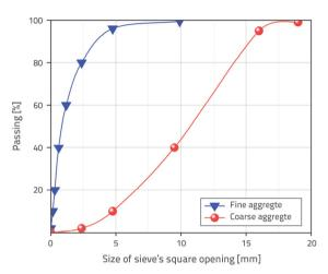
Figure 1. Grading curves of the aggregate
