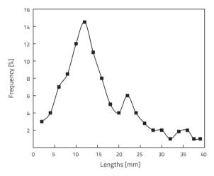
Figure 2. RTSF length distribution frequency diagram
