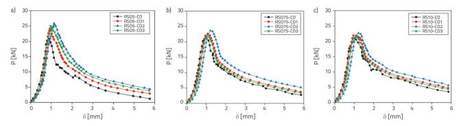
Figure 14. Load-displacement (P-δ) curves for hybrid fibre groups: a) P-δ curve of recycled tire steel fibre 0.5 %; b) P-δ curve of recycled tire steel fibre 0.75 %; c) P-δ curve of recycled tire steel fibre 1.0 %
