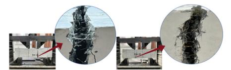
Figure 17. Damage pattern of fibre concrete beam specimens and fibre distribution at fracture
