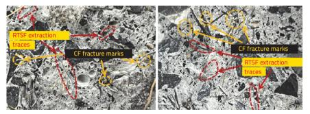
Figure 18. Fibre morphology of fracture surfaces of concrete beams
