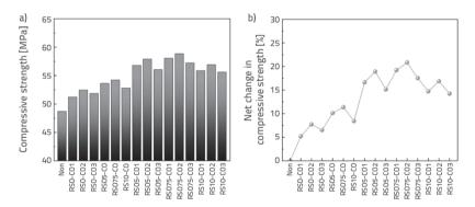
Figure 8. Compression test results: a) Compressive strength; b) Net change in compressive strength
