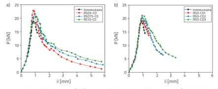
Figure 13. Load-displacement (P-∂) curves of single-doped fibre group: a) Single-doped recycled tire steel fibre; b) Single-doped coconut fibre
