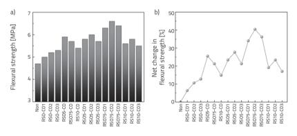
Figure 10. Four-point flexural strength test results: a) Flexural strength; b) Net change in flexural strength
