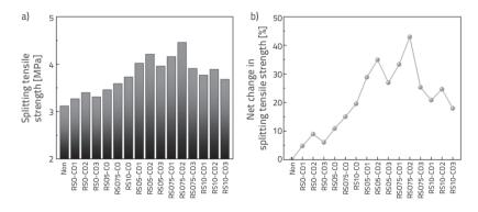
Figure 9. Split tensile test results: a) Split tensile value; b) Net change in split tensile strength
